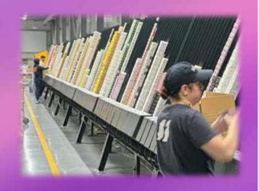
The fully self-operating T-Pick Automated Picking System has a picking capacity of 1800 orders per hour. If we assume that each order contains an average of 25 products, we conclude that it can collect an average of 45,000 products per hour.
